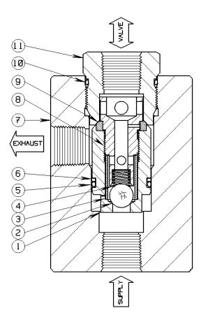
The **13QS38** is a two position, poppet operated control valve assembly. This hydraulic Quick Exhaust valve has a maximum working pressure of **6,000** PSI (413 bar) with **high flow exhaust** capacity. It establishes flow from supply to valve (inlet to outlet) connections to open a Surface Safety Valve (SSV) or Surface Controlled Subsurface Safety Valve (SCSSV) actuator automatically with each application of operating pressure.
