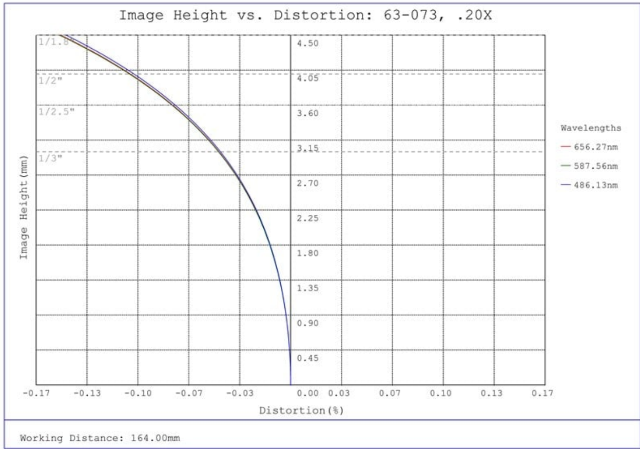
#63-073, 0.20X SilverTL™ Telecentric Lens, Distortion Plot
