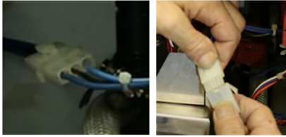
Reconnect high temperature safety cut-out
